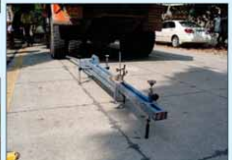
Benkelman Beam deflection Test (BBD)
