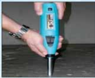
Rebound Hammer Testing
